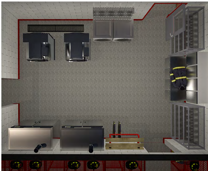
The laundry area of a firehouse should include a washer/extractor that's designed for PPE and a high-temperature residential washer for suitable PPE and personal clothing.
