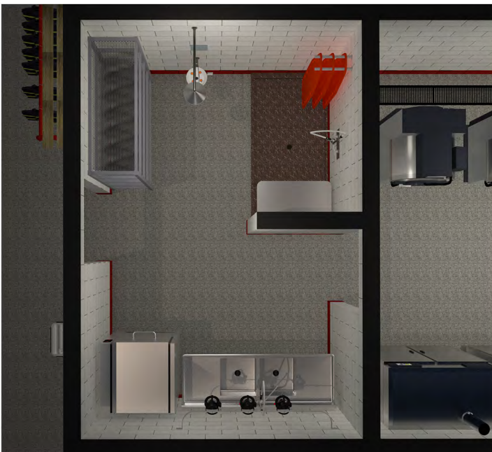
Gross decon area elements are metal shelving, a tub sink and a gross decon chamber.
